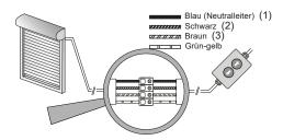
Fig. 5 Connection for assembly cable
